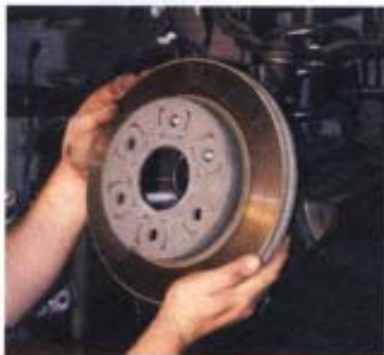
7. The caliper was removed and the rotor was pulled off.
