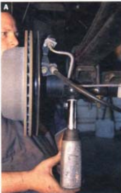
28. A&B With jackstands supporting the axle, the four nuts were buzzed off of the two U-bolts and they, along with the spring plates, were removed.
