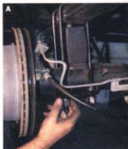
29. Rick raised the lift just enough so that the 4-inch lift blocks would slip in between the leaf and the axle.
