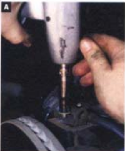
5. Next, the bolts holding the caliper bolt were removed.
