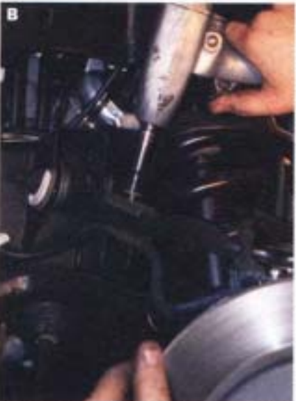
6. A&B The brackets holding the brake and ABS were then removed.
