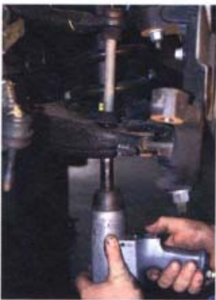
8. Now Rick removed the sway bar endlink from the lower control arm.
