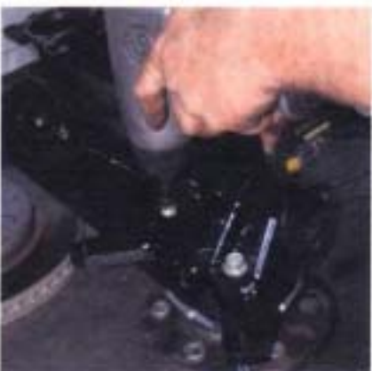
19. ...and the new 4-inch lift spindle bolted up to the hub.
