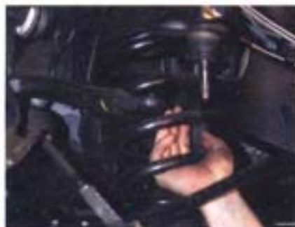
12. The jack was lowered slowly until the coil could be pulled out.
