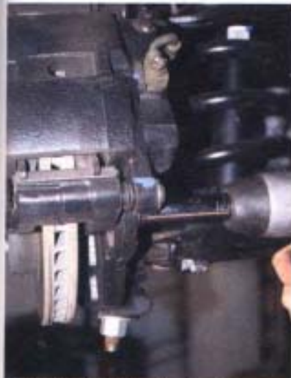
5. Next, the bolts holding the caliper bolt were removed.
