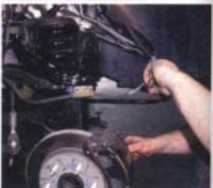
22. The rotor and caliper were then reinstalled onto the hub. A new longer brake hose was supplied, so Rick swapped it out. The brakes were later bled before the truck went to alignment.
