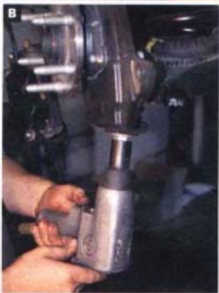
10. A&B The upper and lower ball joint nuts were then loosened up.
