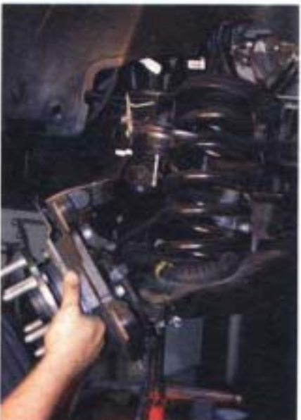
11. A jack was placed under the lower control arm, the spindle was given a few whacks with a 5-pound sledge, and the spindle was removed.
