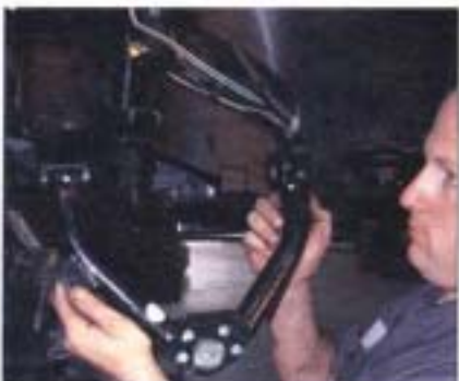
15. Rick assembled the new upper control arms by installing the polyurethane bushings, steel sleeves, grease fittings, and new upper ball joints.
