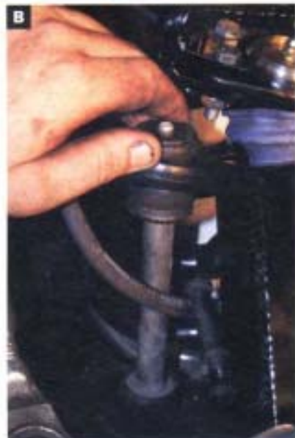
25. A&B Finally, the tie rod end was torqued onto the new spindle and the endlink was reinstalled onto the lower control arm.
